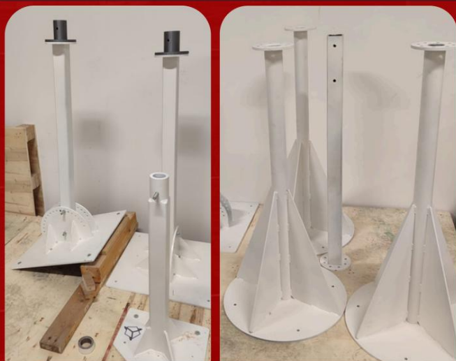
HERE ARE SHOWN THE DIFFERENT TYPES OF PEDESTALS DESIGNED FOR VARIOUS TYPES OF ROOF SURFACES
